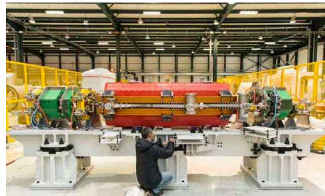
An engineer tests the installation of a vacuum chamber for SESAME
