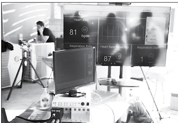
The Defense Ministry announced that its National Emergency Team, together with IAI and Elbit, have developed the prototypes to measure the vital signs of patients, including pulse, respiratory rate and temperature, and pick out patterns that indicate a likely coronavirus infection. (Photo courtesy of Elbit Systems)
