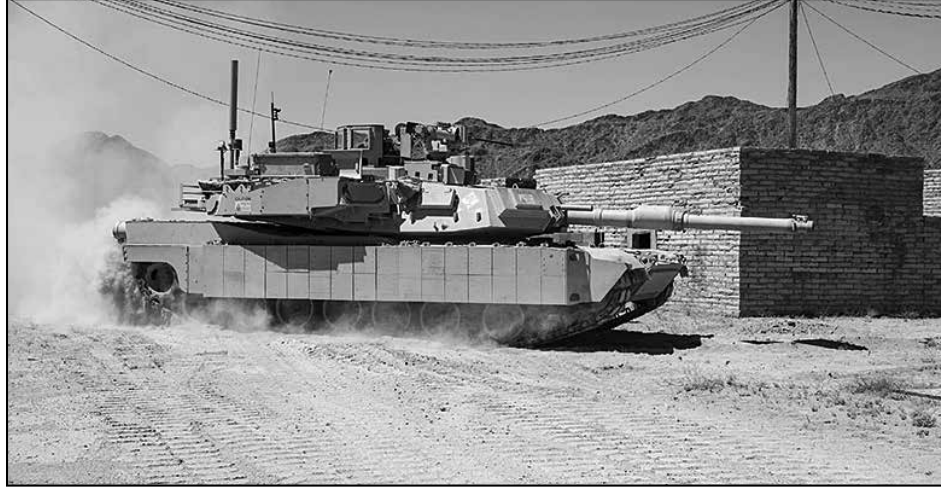
Rafael's trophy system on a U.S. M-1 Abrams tank. (Photo courtesy of Rafael)
